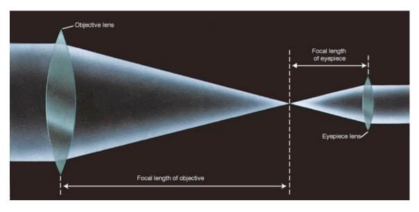
The way it works is quite simple. Light from the star is refracted by its passage through the "Objective Lens" to a point inside the telescope. The light does not stop there! The focus point is simply the point where all the light rays gathered by the objective lens meet. The light keeps going, and is re-refracted by the "Eyepiece Lens" into an image that a human eye can recognize. How much a telescope will magnify an object depends on the "focal length" of each lens.
