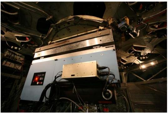
The Project 1640 instrument mounted at the focus of the 200-inch Hale telescope. (AMNH/B. R. Oppenheimer)
