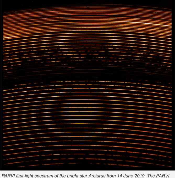
spectral format is typical of echelle spectrometers, with wavelength dispersion along the image horizontal axis, and multiple spectrum orders (the curved semi-horizontal lines) separated (or cross-dispersed) along the image vertical axis. (The PARVI Development Team)
